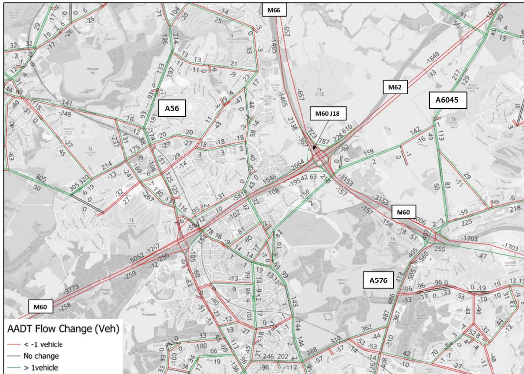
Figure D.1 Phase 1 – DM Traffic Management AADT Flow Change compared to DM (vehicles)
